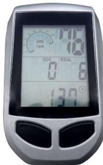
CONSOLE NOTES: The console will display TIME, SPEED, DISTANCE, RPM, and estimated CALORIES
